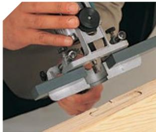
Placing hinges with the ZB93 head.
