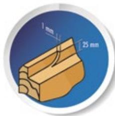
The GR120P is the only planer, together the model CE120P, that permits lateral planing of overlaps of up to 1 mm and a maximum cut height of 25 mm.
