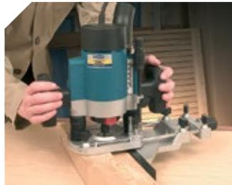
High precision and stability during routing.
