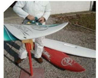
Sanding on materials with several layers of different materials with different hardness and texture.
