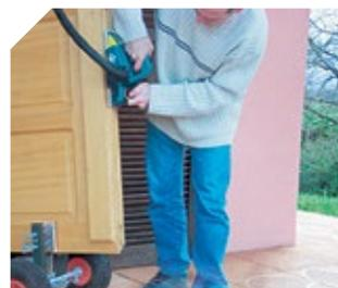
Wheels can be blocked for a stationnary use, so it is possible to work on the edge of the panel or the door.
