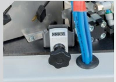
Simultaneous adjustment for the tape thickness, intake guide and gluing roller by a single digital meter.
