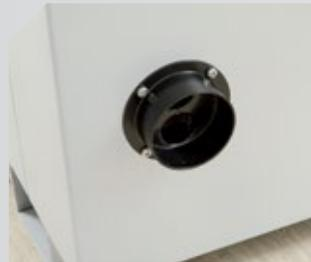
External dust collection for pipes of 100 mm diameter. To be connected to dust collection systems with a minimum air flow of 1000 m<sup>3</sup>/h.
