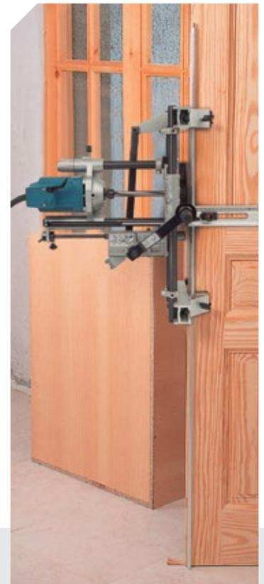
The FC116U incorporates a locking bar, which is fixed to the machine at the height from the ground established for the first mortised door, allowing the mortising of the rest of the doors at the same height without retaking measurements.
