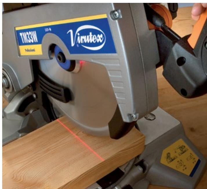
Equipped with a precision laser for guiding the cut. Automatic switch on when the machine starts. With a on/off switch to disconnect it when working on the upper table. The laser device is directly assembled on the saw blade, so the laser beam keeps its precision in any cutting position.
