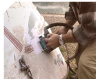
Adjustable to curved surfaces. Specially useful in shipyards.
