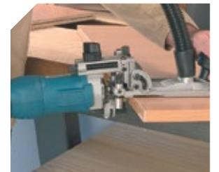
Trimming the edge with the straight bit.
