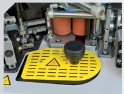
Glue pot with non-stick Teflón® cover. The amount of glue can be also adjusted.
