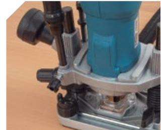
Micrometric adjustment of routing depth. 6 adjustable depth positions for rapid selection of the desired depth.
