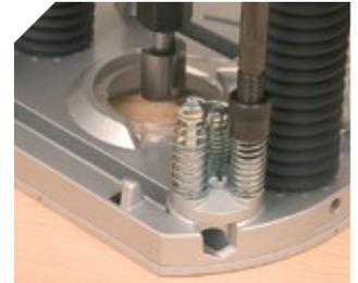
Quick adjustment of routing depth with 3 positions.
