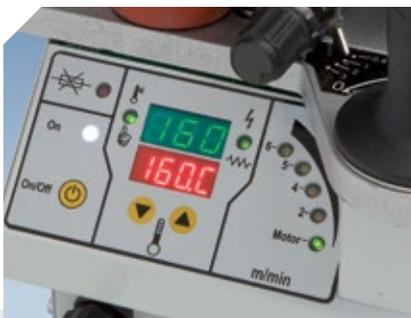
Temperature adjustment (120 to 200°C) controlled by microprocessor for higher accuracy on measurement. Temperature increasing by impulses. Protects the heating elements increasing their working life.
