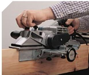
Micrometric fence. For making bevelled edges at different angles.
