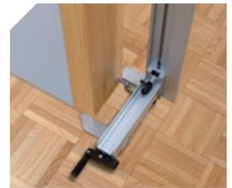
Practice system to fix the machine to the frame and to adjust the cutting width.
