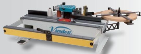
Hot melt glue pot edge bander with automatic rear tape cutting. Foot pedal for curved or shaped pieces.
