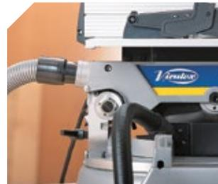
Equipped with a safety mechanism against accidental lowering of the cutting head.
