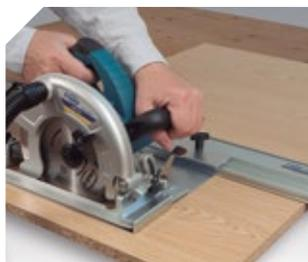
Equipped with dust collection connector.
