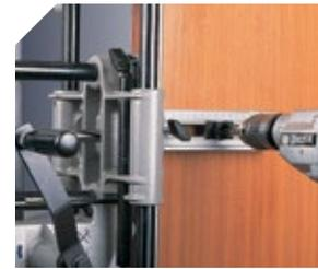
The accessory UT16I allows to take references for drilling the hole for the handle and key cylinder.
