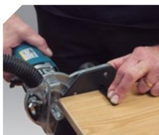
Precise guide for corner trimming (ref. 5600060).
