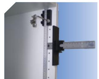
Drilling for placing invisible hinges.
